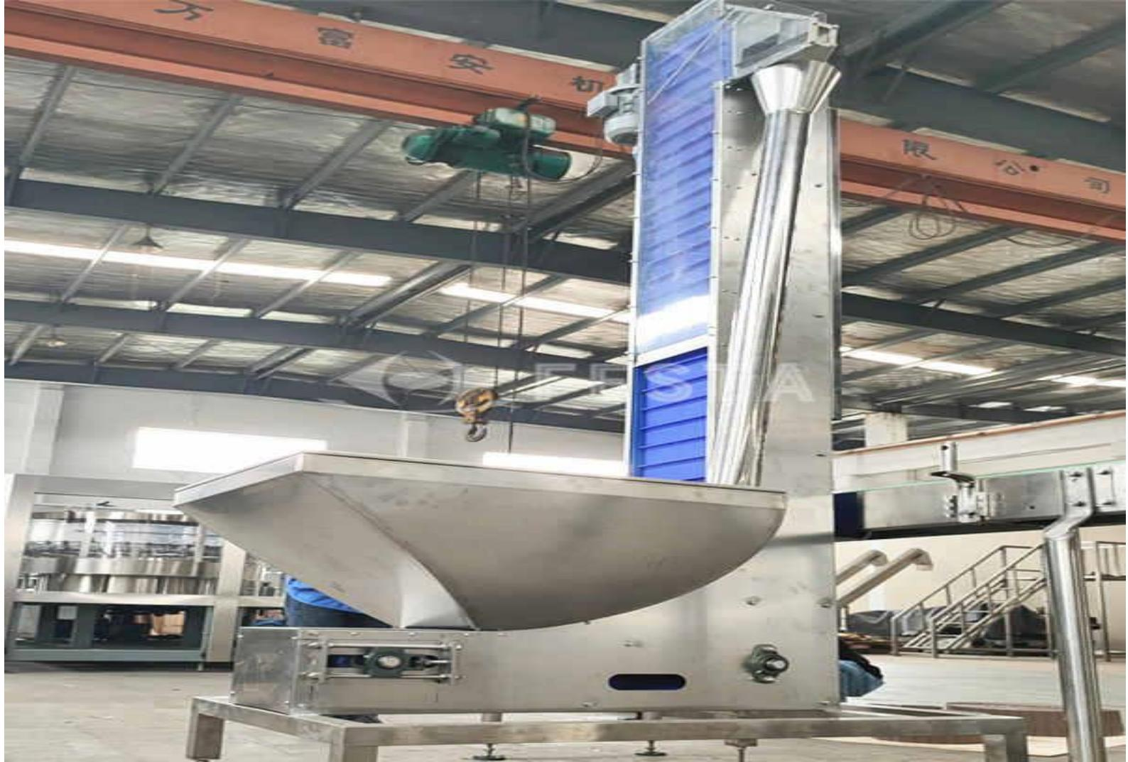
Here are the detailed specifications and descriptions for a **Cap Elevator** and **Cap Orienter**, which are essential components in automatic bottle capping lines. These systems ensure continuous feeding and correct orientation of caps before capping.
